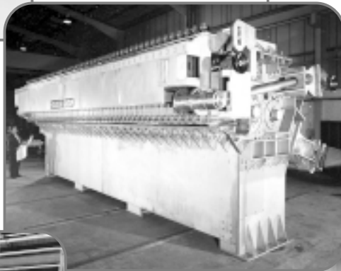
Headbox Adjustment on Paper Machine
